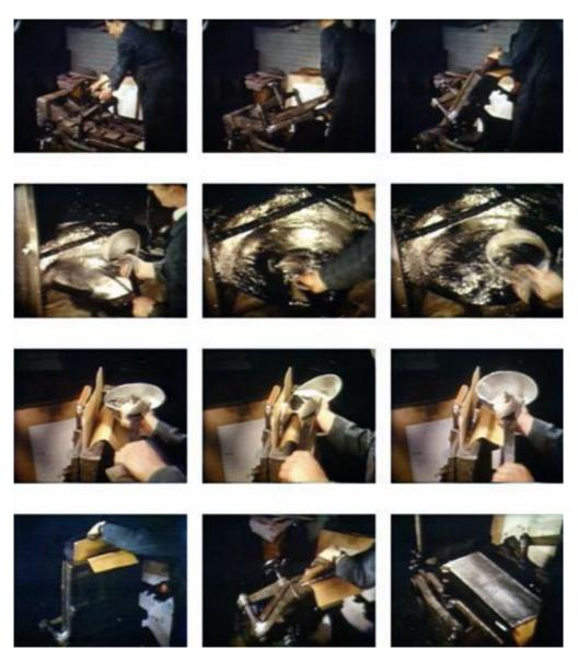
Casting a stereotype plate: 1–3 closing the casting box and moving it into a vertical position, ready for casting; 4–6 filling a ladle with molten type metal; 7–9 pouring type metal into the casting box; 10–12 the casting box is returned to a horizontal position and opened to reveal the cast metal plate.
