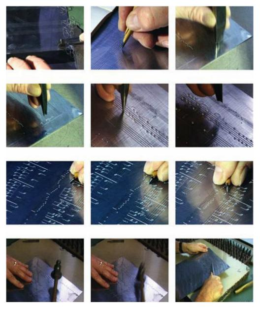
Engraving sheet music: 1–2 Preparing the plate – staves being cut with a five-pronged rule and sketching out the notation with a steel nib; 3–6 Using steel punches to add notation into the plate; 7–9 Cutting a slur into the plate freehand; 10–11 Smoothing the reverse side to reduce the tension in the plate; 12 Marking a sign for correction with a pincer.
