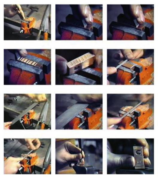
Applying a Benday tint to a plate: 1–2 stopping out areas not to have the tint applied; 3 selecting a Benday screen; 4–6 inking the screen; 7–8 fixing the screen to the shading machine; 9–12 transferring the Benday tint onto the plate using a burnisher.
