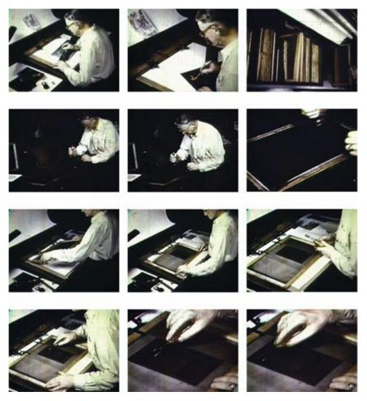
The final stages of justifying a matrix: 1–5 Botching the matrix (widening it in order to correct the positioning of the character on the body of the matrix); 6–8 Filing a notch on the back of the matrix; 9–10 Filing leather grooves on the back and then the front of the matrix; 11 Punching identifying marks into the matrix; 12 The finished matrix ready for casting.
